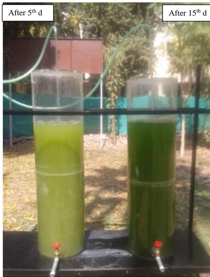
**Fig. 4:** Cultivation of SBC 2 at outdoor conditions for the removal of pollutants from dairy wastewater
